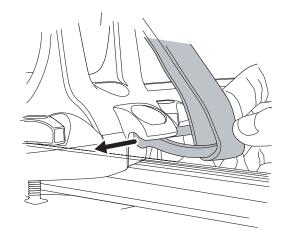
7. Rotate the buckle up to lock it into the base. Repeat this step at the remaining bases.
