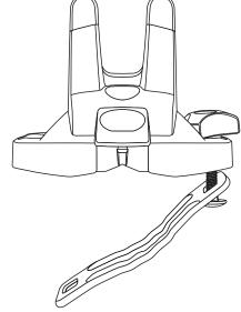
2. Position the base on the crossbar. Loosely install a bolt and knob as shown.
